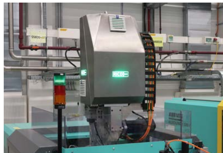
Electric handling systems are low-noise, precise, fast and interface-compatible, as well as space-saving
