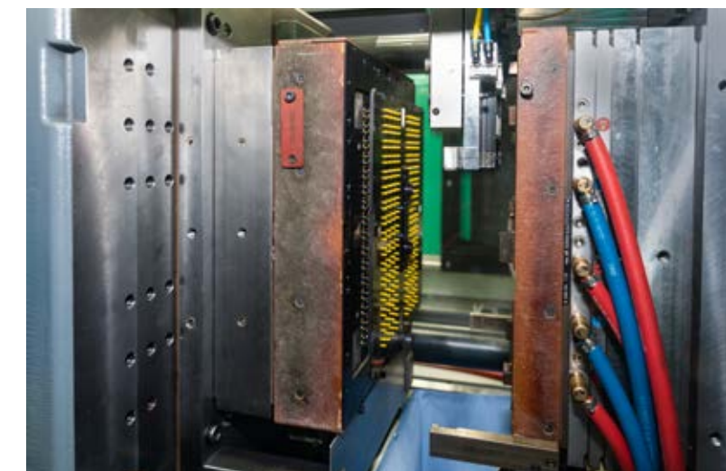
256-cavity mold for the production of single wire seals
